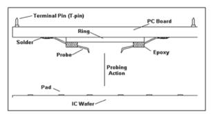
Figure 1-3: Probe Card and Wafer
