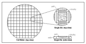
Figure 1-1: Integrated Circuit Wafer
