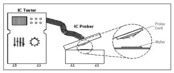
Figure 1-2: IC Tester and Prober (with probe card and wafer)
